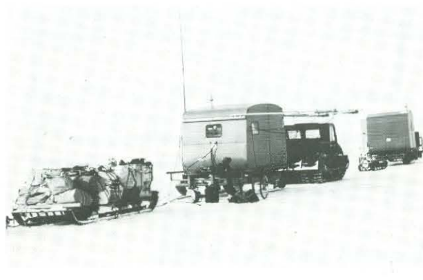
PLATE 2. The Geophysical Caboose with supporting booms for echo sounder folded dipole. The motor-generator set is visible at the rear of the caboose
