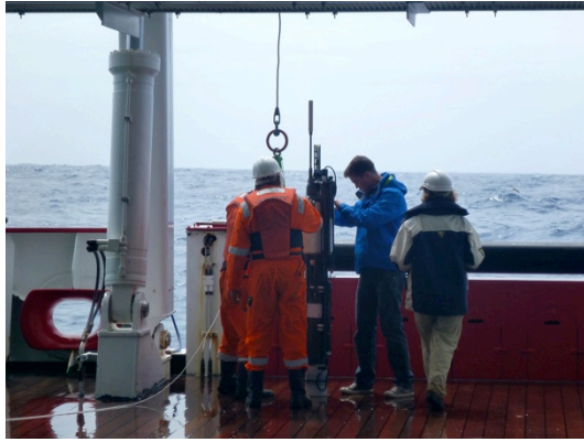
Figure 3: Oceanographers and ship's crew readying to deploy an argo float. Photo: C. Hansen.
