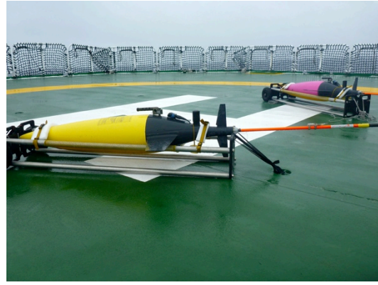
Figure 4: Two underwater gliders being calibrated in the helicopter deck of the Agulhas II. Photo: C. Hansen.
