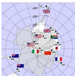
Coverage and national associations of the 11 SuperDARN radars in the Southern Hemisphere. The beam of each radar scans an area of about 4 million square kilometres. The overlapping of the beams permit the estimation of both the speed and the direction of travel of ionospheric structures over the South Pole. A similar network is monitors ion flow over the North Pole.
