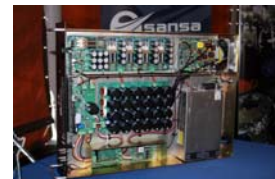
One of the T3 Transceiver units of the new HF Radar at SANAE-IV. All 16 the units for the HF Radar were built and tested at SANSA Space Science in Hermanus.
