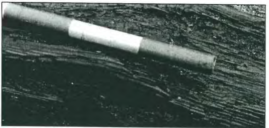
Ship's frame with iron bolt. Scale = 10cm divisions
