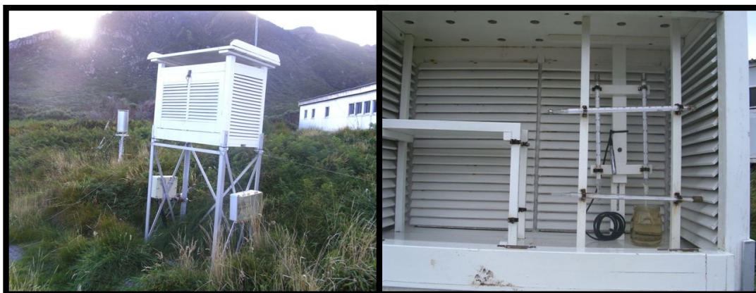
Stevenson Screen: Dry and Wet bulb thermometers at the back and the Maximum and Minimum Thermometers in front.
