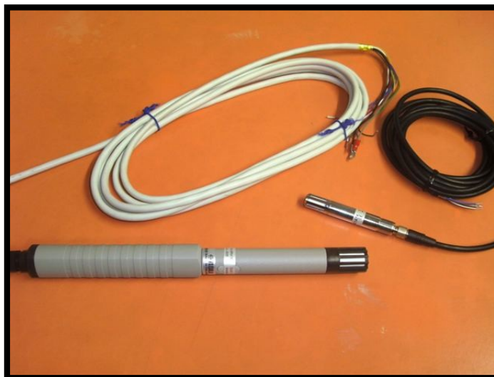
Viasala Intercap temperature /humidity Probe HMP 50 YA and the Viasala HMP 45 D temperature/humidity transmitter
