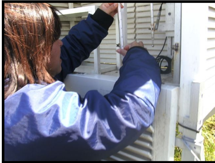
Observer resetting maximum and minimum thermometers
