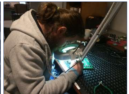
Figure 12, 13 & 14. The chips in question. Travis concentrating and working carefully, replacing the chip on the broken modem card.
