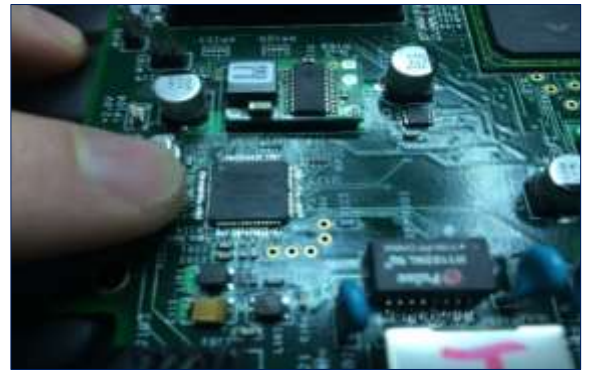
Figure 11. The chip in question on the broken modem card.
