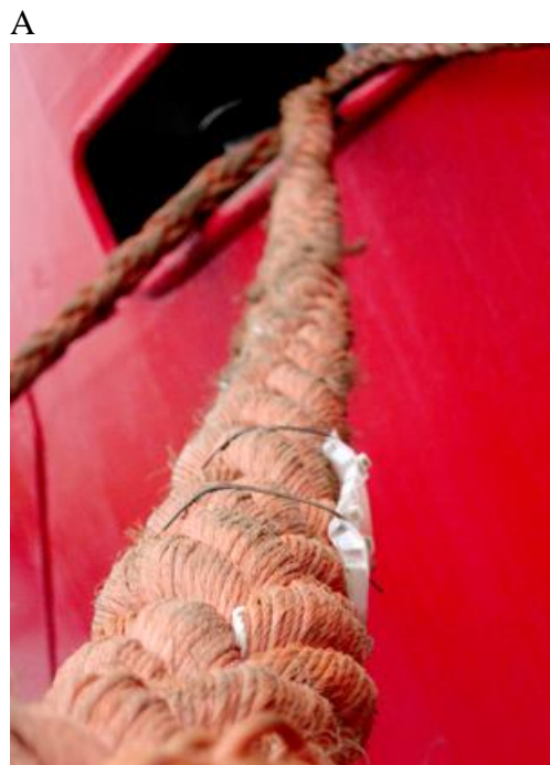
Figure 1. Glue-board inappropriately attached to a hawser, probably due to the rope twisting while under strain.
