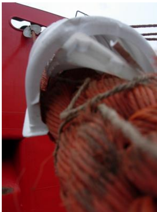
Figure 2. Glue board inappropriately attached, allowing rodents access.
