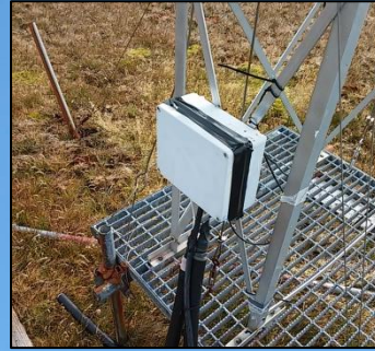
Junction box connecting wind, rain and temperature sensors
