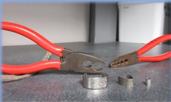
Ringing pliers for rings to fit all kinds of birds: Wandering Albatross (left), Sooty Albatross (middle), Storm-petrel (right)
