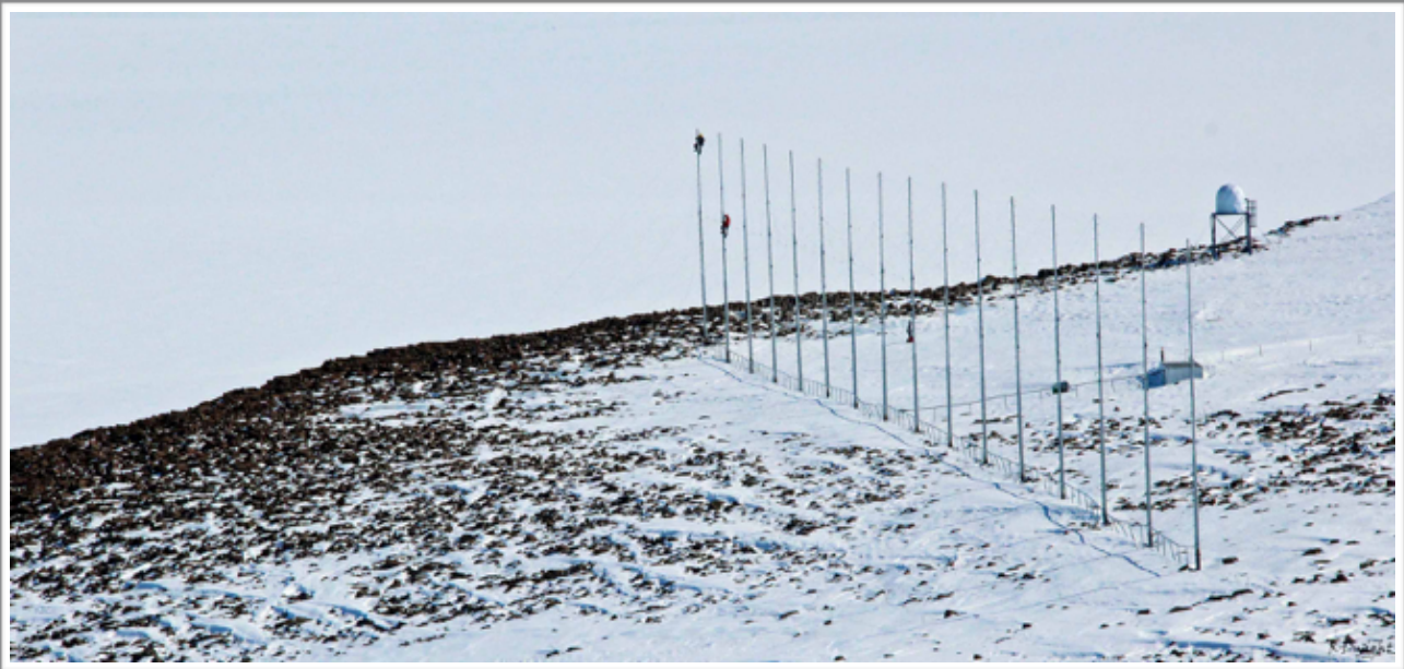
2. The SuperDARN HF Radar has a main array with 16 antennas and a secondary array with 4 more antennas.
