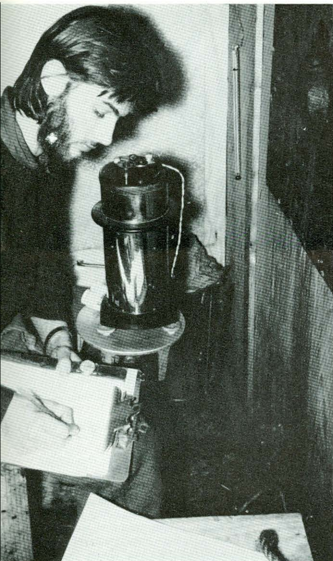
Derek Sharwood at the substation, operating the gravimeter by which the change in gravity, indirectly indicating the degree of up and down movement of the ice-shelf, was determined.
