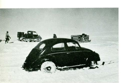
The modifications made to the Volks-wagen to enable it to travel on snow and ice are clearly visible in this photograph. (Photo—Department of Transport.)
