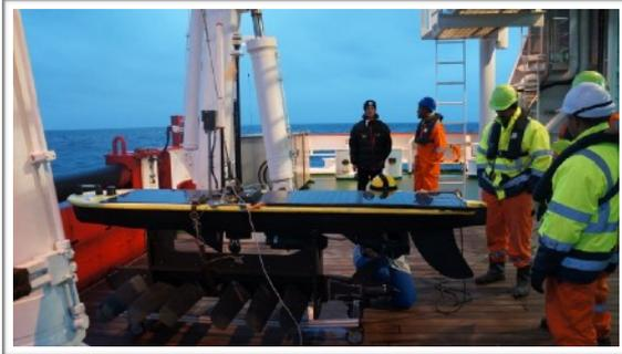
**Wave Glider and Slocum Glider:** These were the two yellow things that we waited so long for...The wave glider looks like a little boat which has a 7m umbilical which is connected to some fins. The glider sits on the surface of the water and then, through wave action on the fins, is pushed along its path. It collects surface data including temperature and
