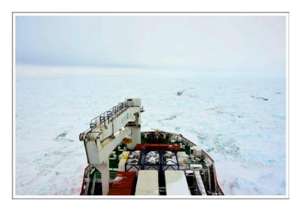
Other than the fuel bunkers there are also several holds for cargo. These are used variously for big shipping containers, vehicles (being returned to the base after being serviced in SA), petrol drums for the snowmobiles, and construction equipment being used at the base for the upgrades. There are several cranes of different sizes to move all this onto the ship and also around the ship.
