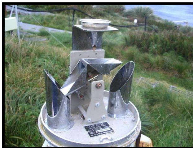
Tipping buckets underneath the inner receiver funnel
