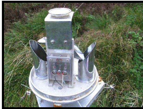
Reed Switch at the back of the tipping bucket
