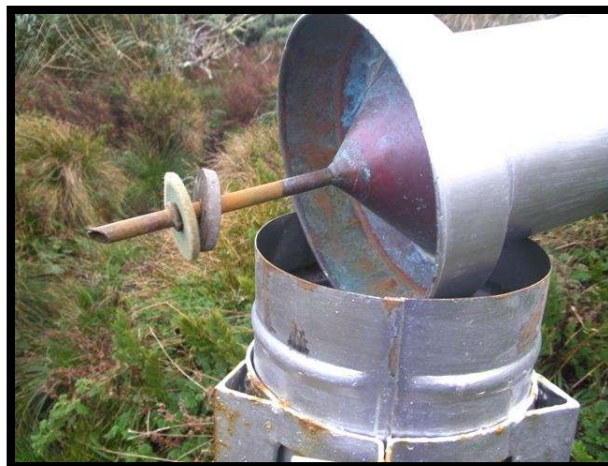
An evaporation disc and with felt underneath
