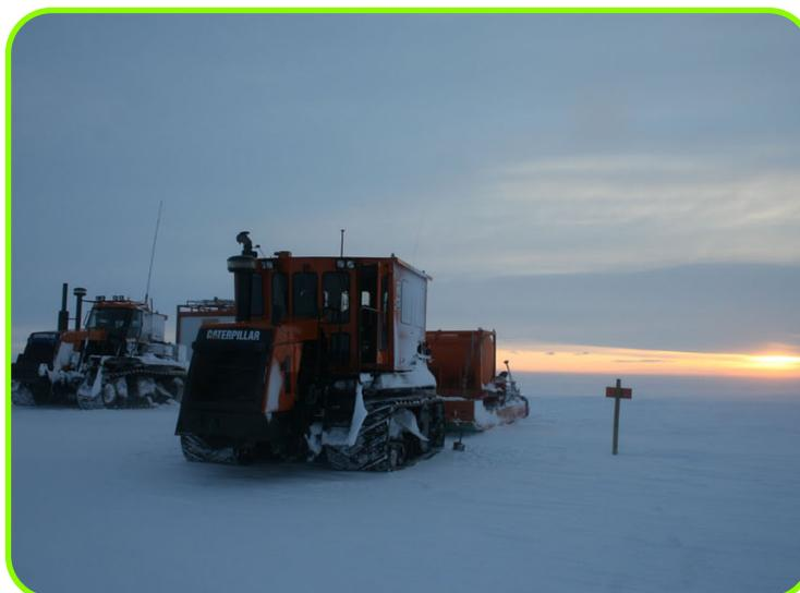
Each year the overwintering team is tasked with inspecting the fuel depot where some of the programs' diesel bowsers (diesel tanks on sledges) are stored. At the end of each takeover large ramps are dozed and the sledges pulled on top with a winch. This is to ensure that the snow buildup does not bury the sledges entirely.
