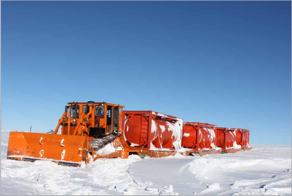
The blade-dozer pulling approximately 100 tonnes en route to the Winter Depot
