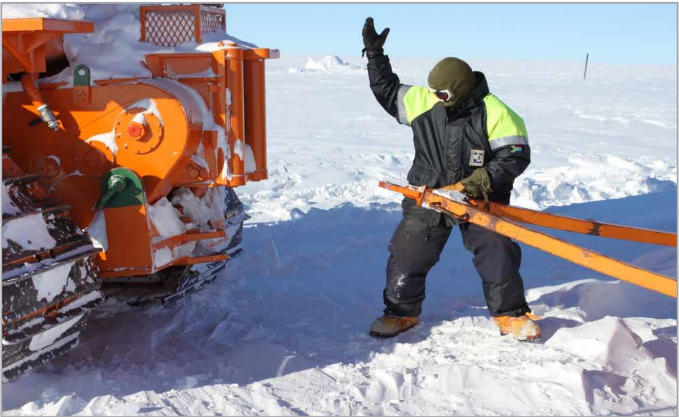
Connecting a cargo sled's A-frame to the back of a bulldozer
