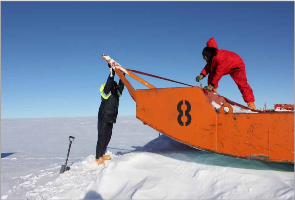
An empty cargo sled on its ice throne in the Winter Depot - two S49 team members are tying up the A-frame, so that it will not be buried under ice during the winter.
