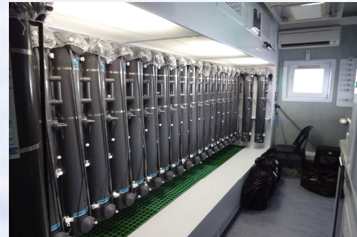
Figure 1: Class 10 trace metal clean sampling container-laboratory on board SA Agulhas II
