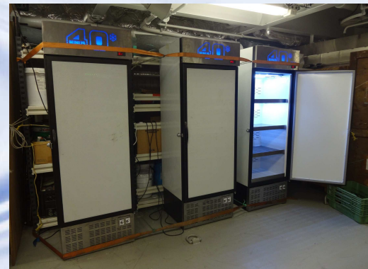
Figure 4: Light and temperature modulated incubators used for bioassay experiments
