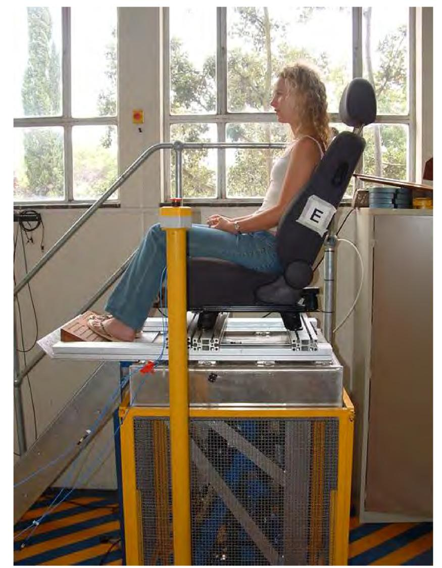
The BS ISO 2631-1:1997 standard does provide a guideline for the assessment of comfort, however the standard is intended for the analysis of vibrations without shocks. Since the vibration during the voyage often included shocks, the comfort needs to be further investigated by a laboratory study.
