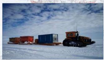
Figure 3. CAT train: a Challenger pulling a loaded, 6-meter container and 2 x 25 000 litre polar diesel bowsers.
