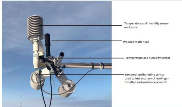
Figure 1A. The automatic weather station set-up exposed to the Antarctic atmosphere. The weather station is installed 2m from the ground and is at an elevation of 865m above sea level.
