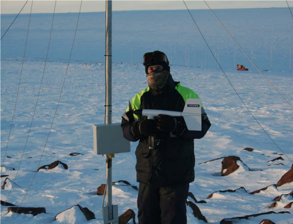
The ‘metkassie’, the anemometer and the mast (Hint to those readers that don’t know what an anemometer looks like: our peace-loving meteorologist isn’t cradling a cruise missile in his arms, we promise)
