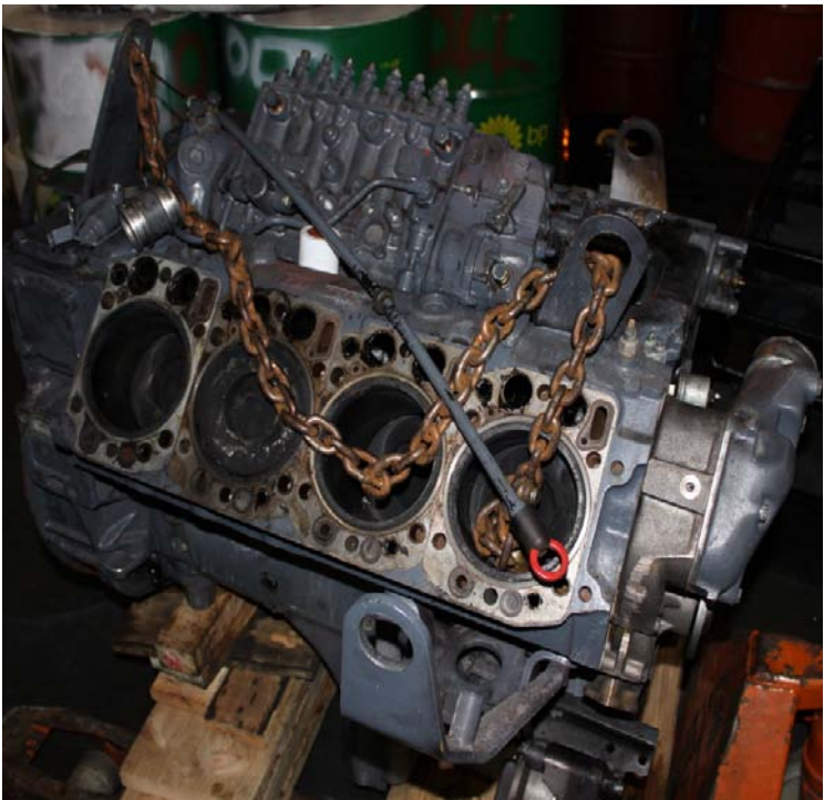
The engine of Genny 1, showing four of its eight massive cylinders.
