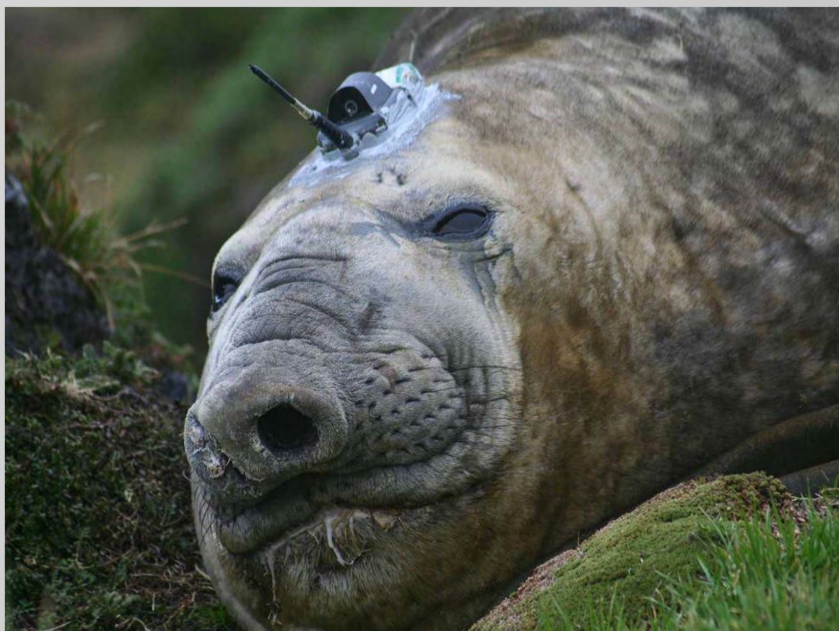
FIGURE 1. Adult male SES fitted with a SMRU satellite tracking device. This device collected temperature and salinity at various stages during the seals dive.
