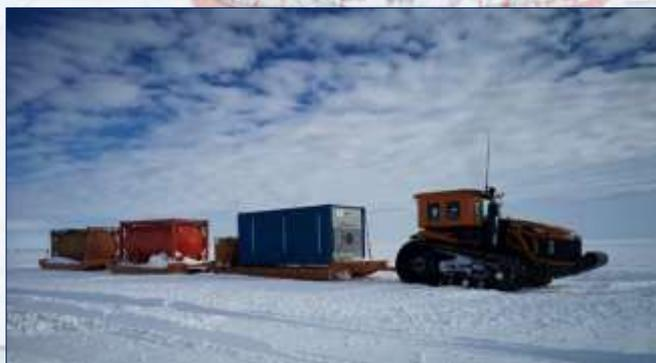
Figure 3. CAT train: a Challenger pulling a loaded, 6-meter container and 2 x 25 000 litre polar diesel bowsers.
