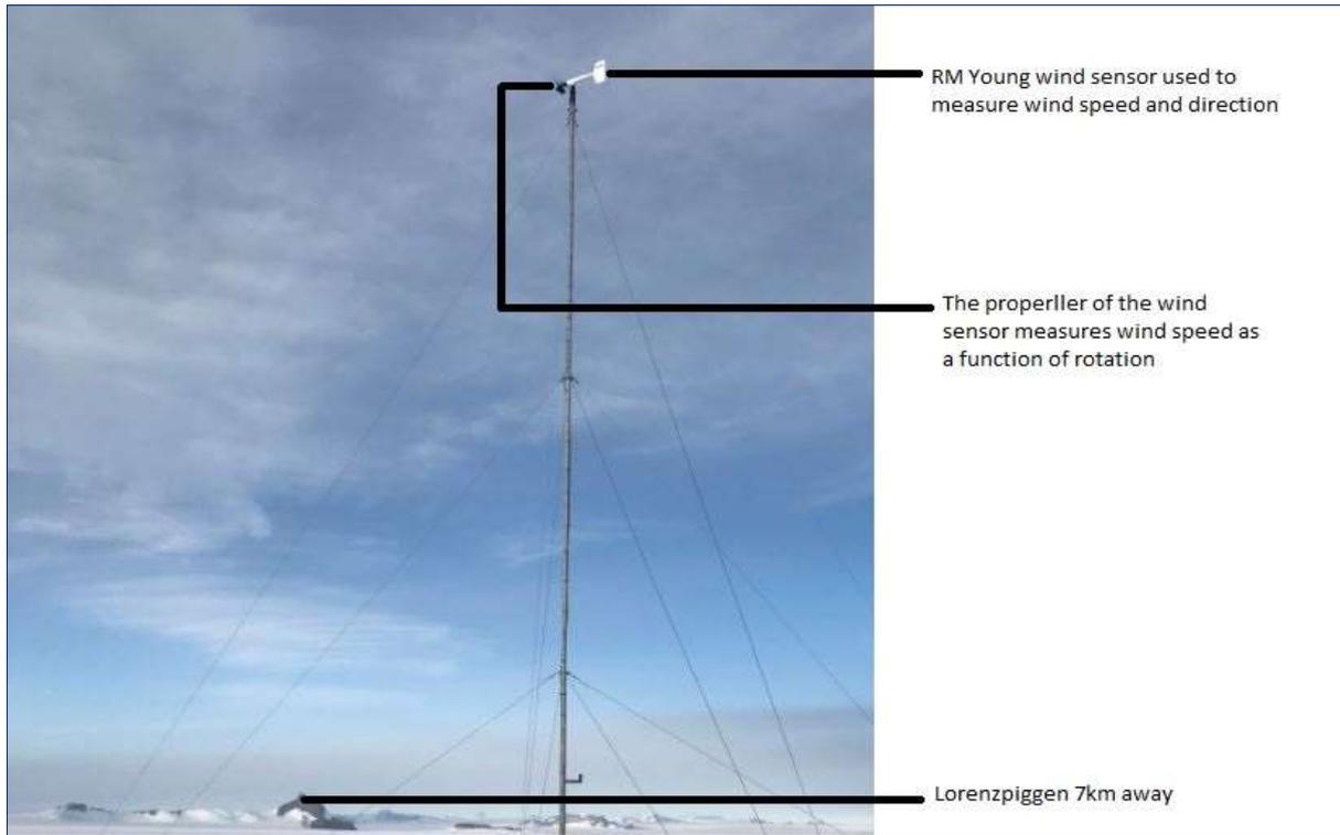
Figure 1B. An anemometer installed 10m clear of the ground, used to measure wind speed and direction. The propeller always faces in the direction from which the wind is blowing, i.e. as depicted here East of South East.
