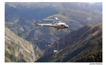
**Figure 4.** Typical helicopter and bait spreader bucket used in aerial rodent eradication projects.
